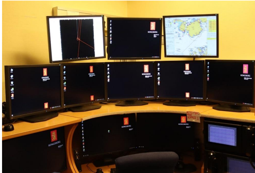
Figure 7: RNoNA ship-handling simulator control room, instructor station.
