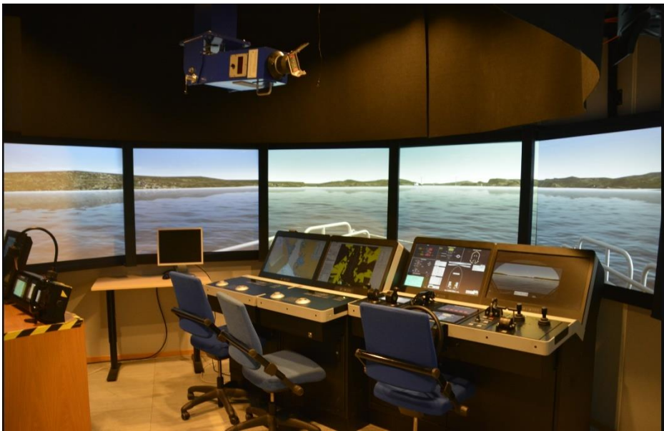
Figure 6: RNoNA ship-handling simulator small bridge
