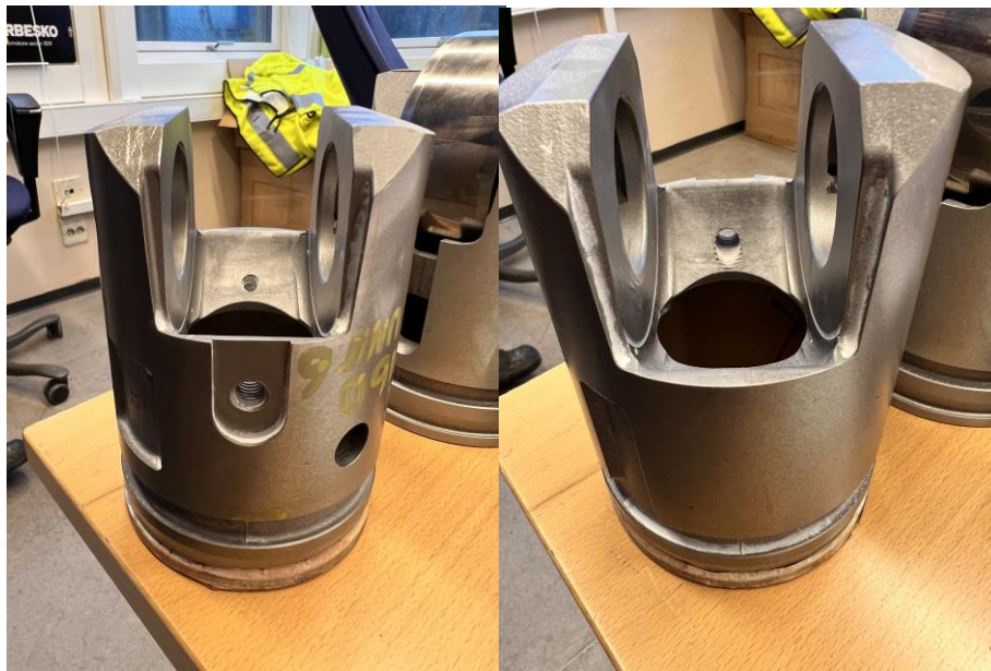
Figure 14 The real-life model with the strained areas visible
