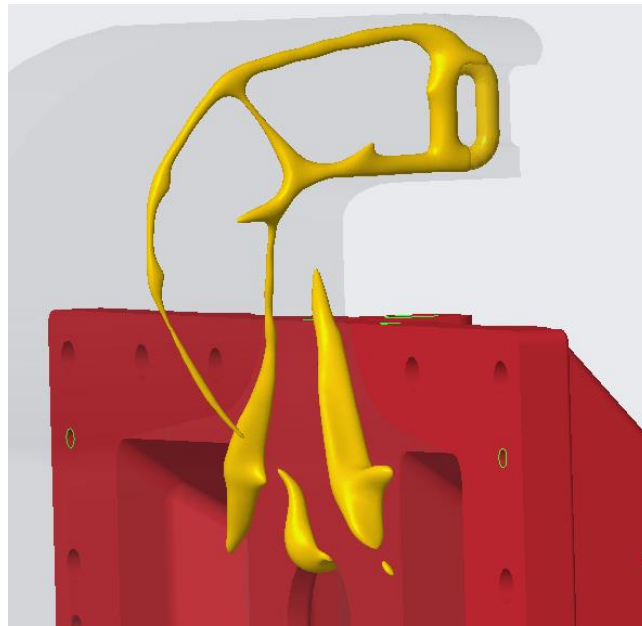
Figure 41 Lifting tool Design 1 improved unsuccessful with 316L
