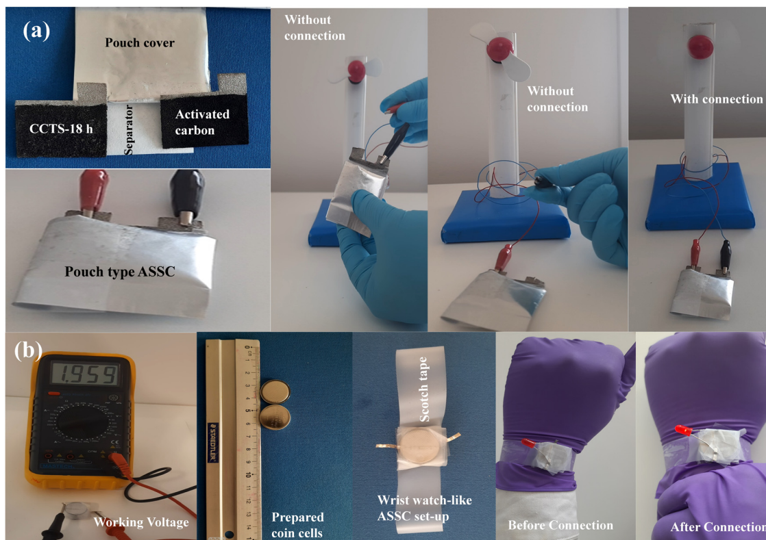
Fig. 11 (a) Working model of the pouch-type ASSC and (b) photograph of the assembled wristwatch-like coin-cell ASSC.
