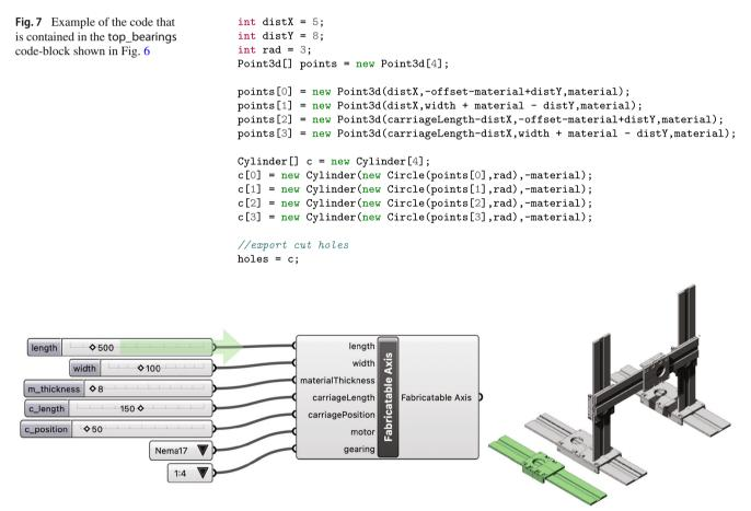
Fig. 8 Interaction with the Fabricatable Axis model. By changing the input parameters of the model, users can create instances of the model and arrange them in Rhino
