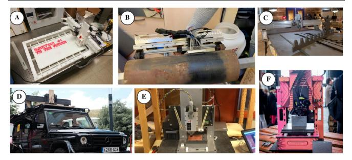
Fig. 14 Examples of machines built with the Fabricatable Axis. **a** Pen-Plotter, **b** Pipe-inspection robot, **c** Large-Format CNC mill, **d** CNC mill on top of a Gelendewagen, **e** PCB milling machine, F. 3D printer with silk screen decals
