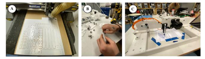
Fig. 13 In A the parts for the 2-axis pen-plotter is cut using a CNC milling machine at a local Makerspace. B shows the assembly process of the machine. In C the completed pen-plotter is being used to draw line art on paper
