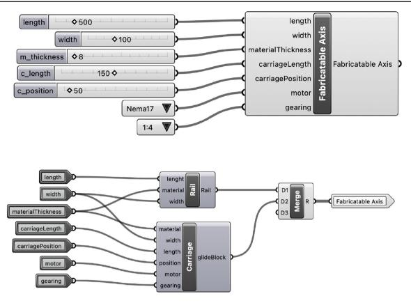
Fig. 5 Top figure shows the Fabricatable Axis top-level cluster in Grasshopper. Bottom figure shows the top-levels sub-clusters; Carriage and Rail. These clusters are merged into the output of the Fabricatable Axis
