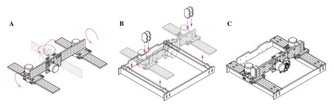
**Fig. 12** Process of designing 2-axis pen-plotter using the Fabricatable Axis. The model is used to generate 3 different actuators. The actuators is then put in a machine composition by translating and rotating them in
