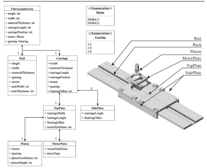
Fig. 4 Domain-model of the Fabricatable Axis
