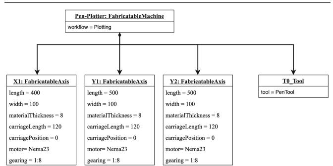
Fig. 11 Object diagram of the Pen-Plotter
