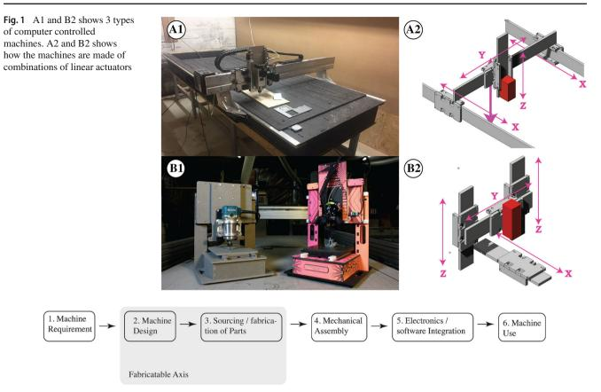
Fig. 2 The steps to go from a machine requirement to a machine implementation
