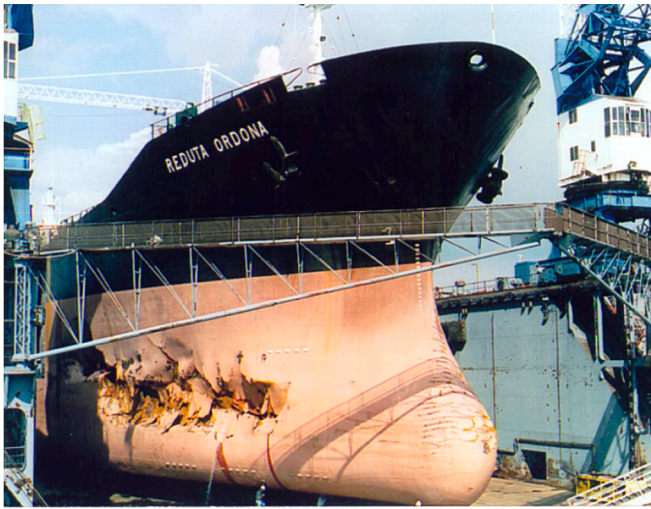
Fig. 1. The bulk carrier “Reduta Ordonea” collided with a growler in Hudson Strait on its way from Poland to Churchill, Manitoba, July 21, 1996 [1].
