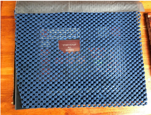
Fig. 2 Example of adaptation of technology by seafarers. All the available alternatives for managing window wipers except the one they need (start/stop all wipers) has been covered
