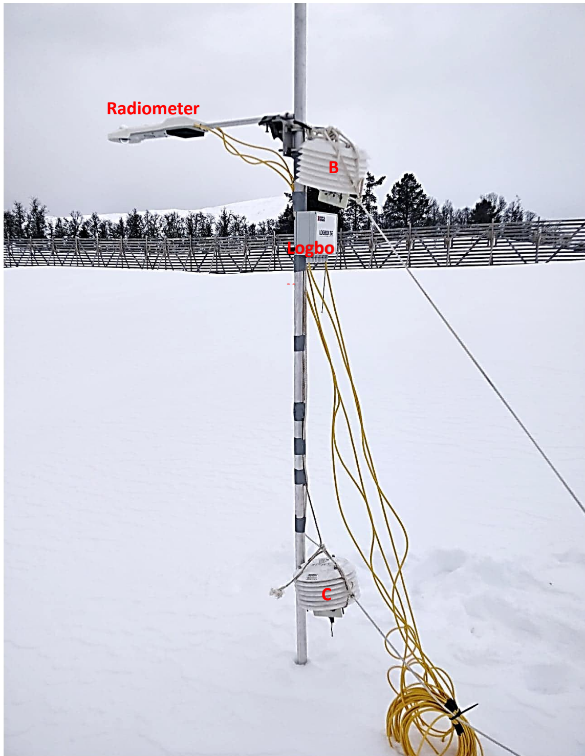
Figure 8 Setup of logging equipment looking west. CNR4 Net Radiometer on the left connected to a Logbox SE. Two Tinytag temperature loggers at about 10 cm (logger C) and 150 cm (logger B) from the snow surface, inside white sun shields. Wiring and Tinytags are tied to the north side of the pole to limit shading effects on the radiometer. This photo was taken the 7 th of April, right before dismantling.
