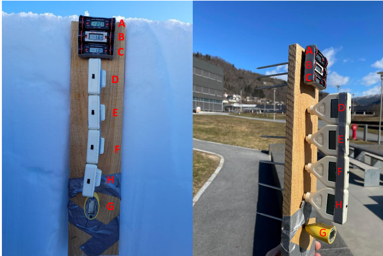
Figure 11 The "Thermoplank". Eight thermometers mounted to a plank to make temperature measurements in a snow profile more efficient. Each thermometer is labelled with a letter to distinguish them in the data.
