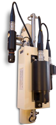
Figure 28: CTD sonde as used for the hydrographical measurements in the tributary fjord basins. Reprinted from SAIV A/S (n.d.).
