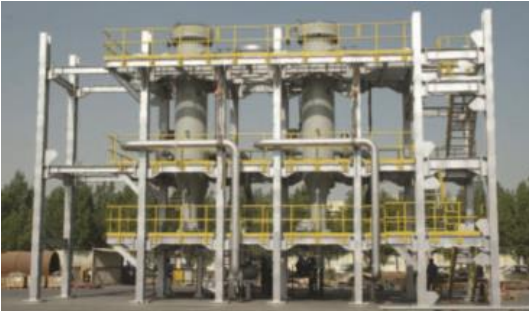
Figure 21: Cyclone filter separator layout [22]
