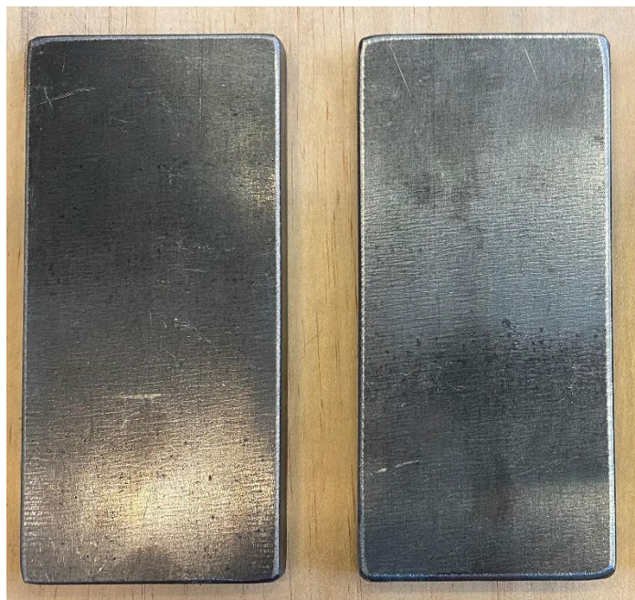
Figur 25: Testplate, ubehandlet stål
