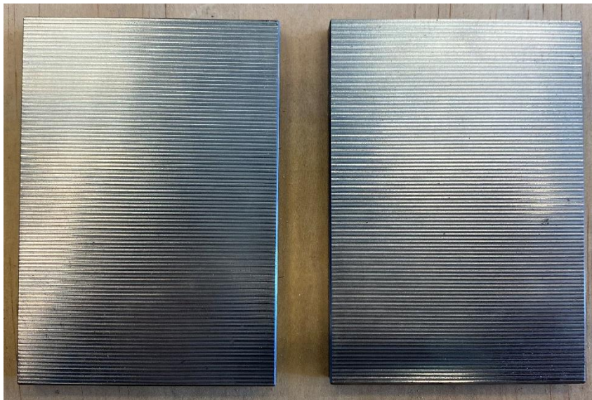
Figur 23: Testplate, Ra = 6,3 \mu\text{m}
