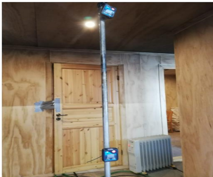
Figure 6: Orientation of gas measuring device at different heights during the experiments (picture taken with RNE-L21-HUAWEI)
