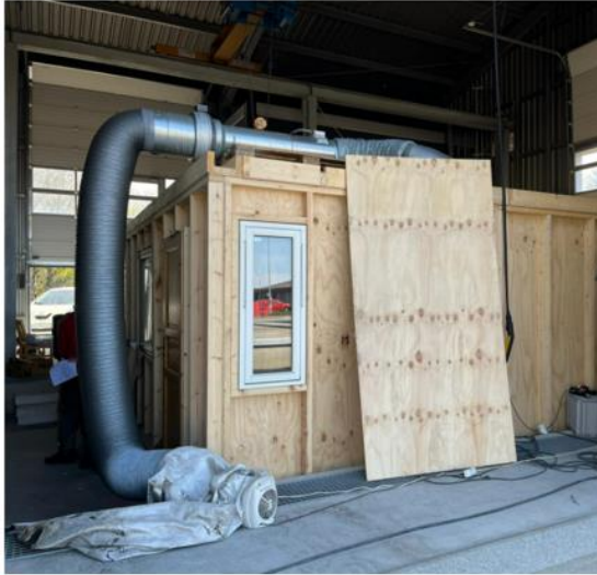
Figure 8: Ventilation system installed in the apartment at the Hall of Flame
