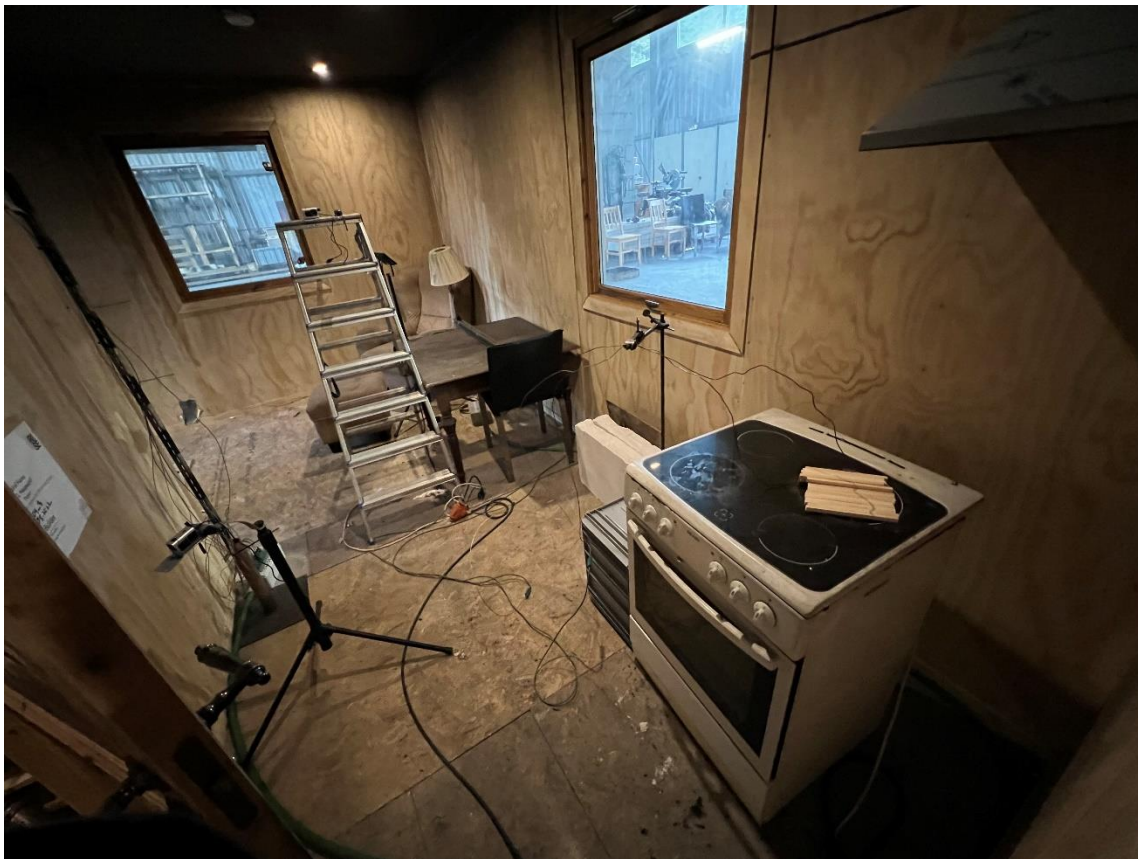
Figure 4.7: Experimental setup of Smoldering Wood Fire (with ventilation System)
