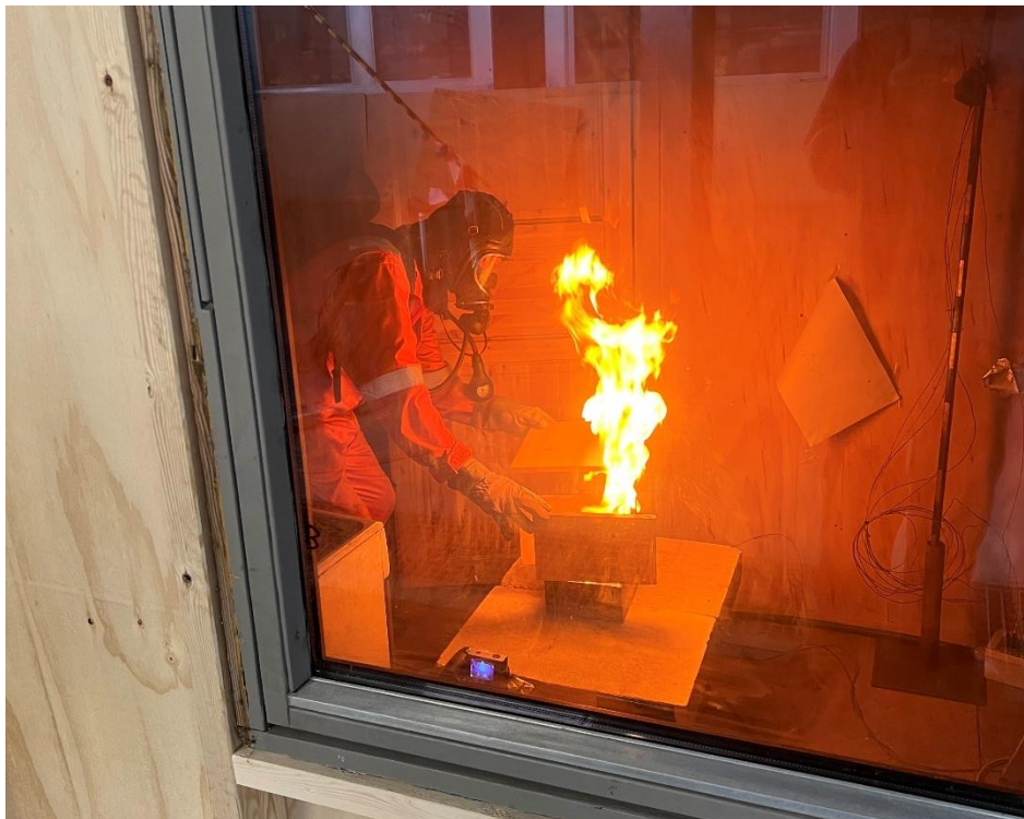
Figure A6: Testing further development of fire (Test Number 204_4)
