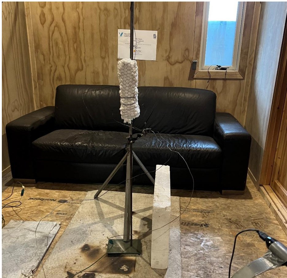
Figure 4.4: Experimental setup of Glowing Smoldering cotton Fire (With no ventilation)
