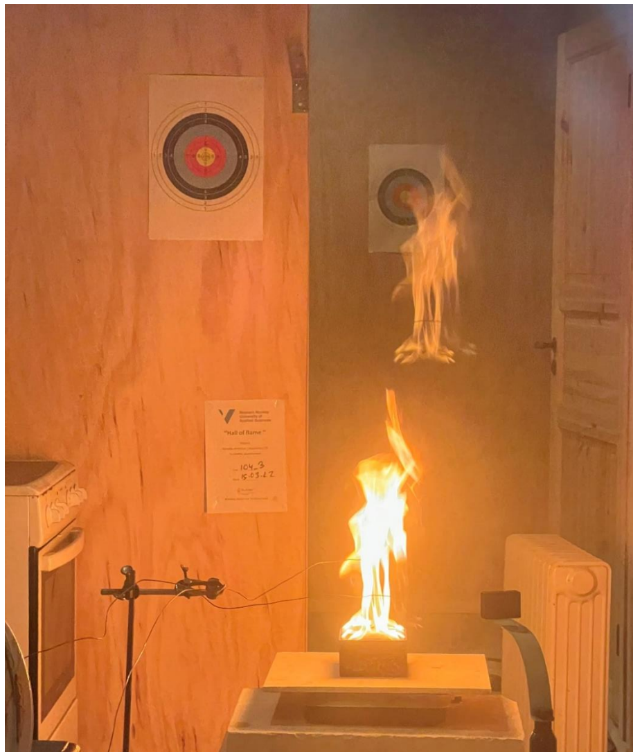
Figure 4.6: Experimental setup of Burning Heptane (With no ventilation) (104_1 to 104_4)
