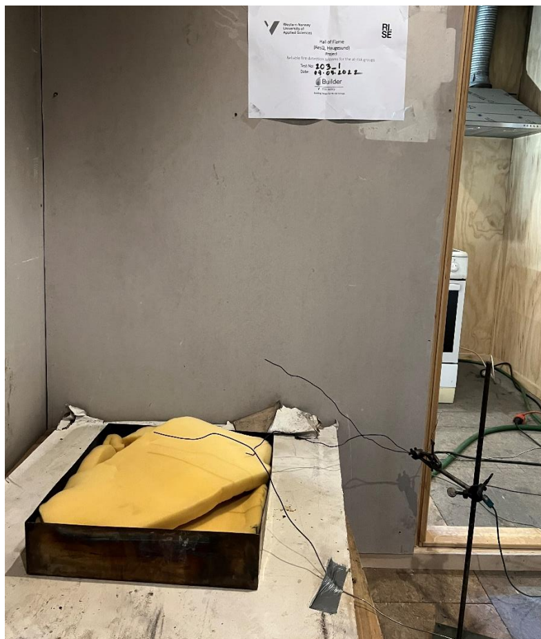
Figure 4.9: Experimental setup of Burning Polyurethane (With ventilation system)
