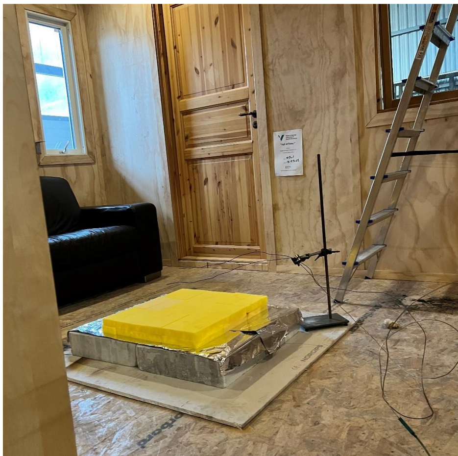
Figure 4.5: Experimental setup of Burning Polyurethane (With no ventilation) (103_1 to 103_4)
