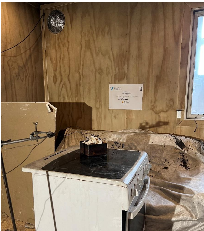
Figure 4.8: Experimental setup of Slow Smoldering Cotton Fire (With ventilation System) (202_1 to 202_4)
