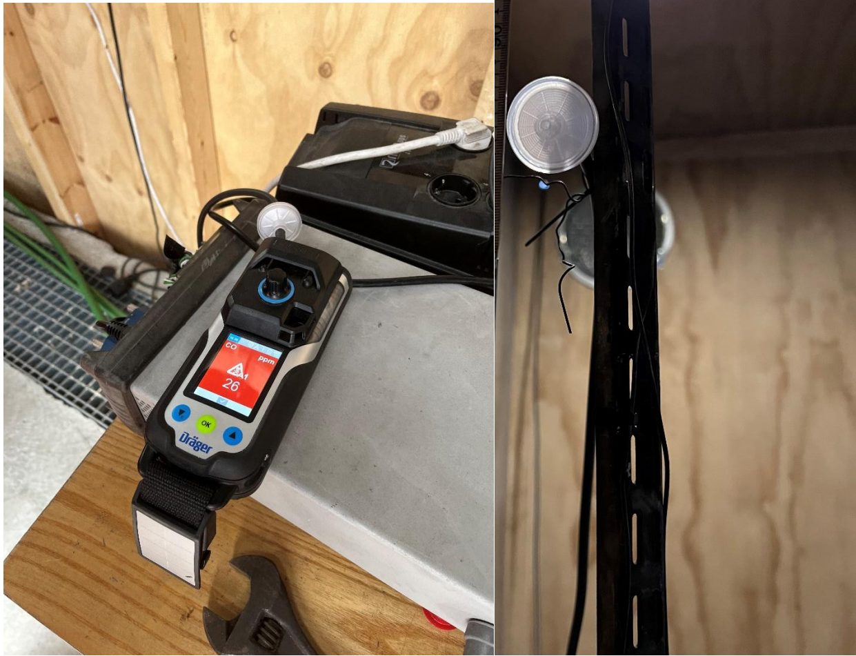
A11: Dräger X-am 8000 gas Detector and air sample inlet inside apartment
