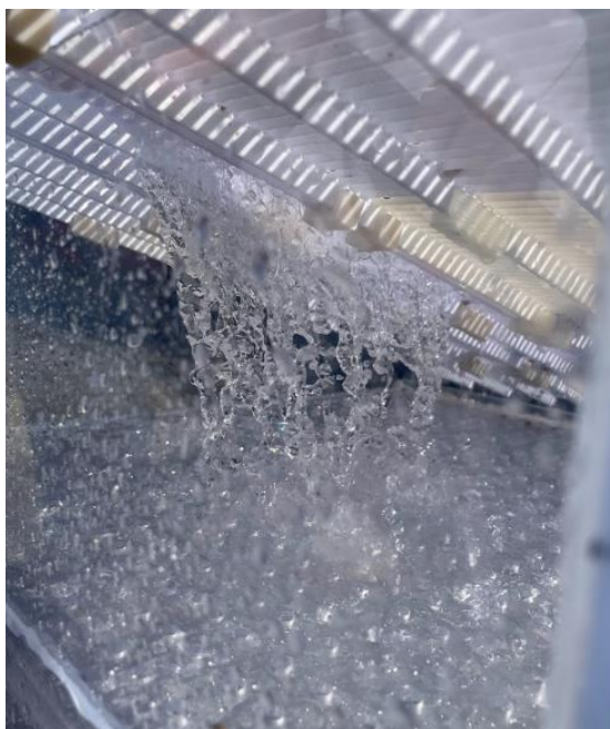
Figur 38: Vannfordeling under wedge wire
