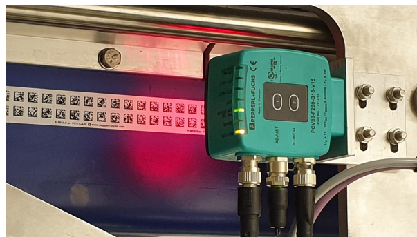
Figure 4.4: QR scanner on the carriage.
