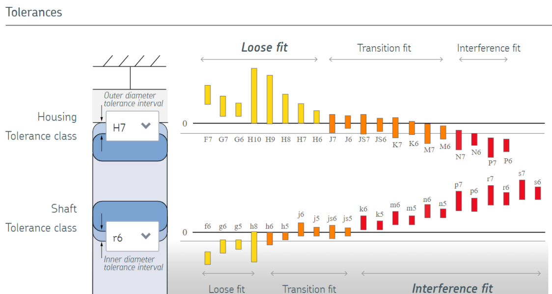
Figure 3.12: ISO 286-1 system for tolerances [36].
