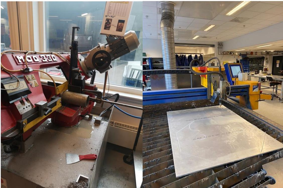
Figure 27 - Hacksaw (Left) and CNC Plasma Cutter (Right)
