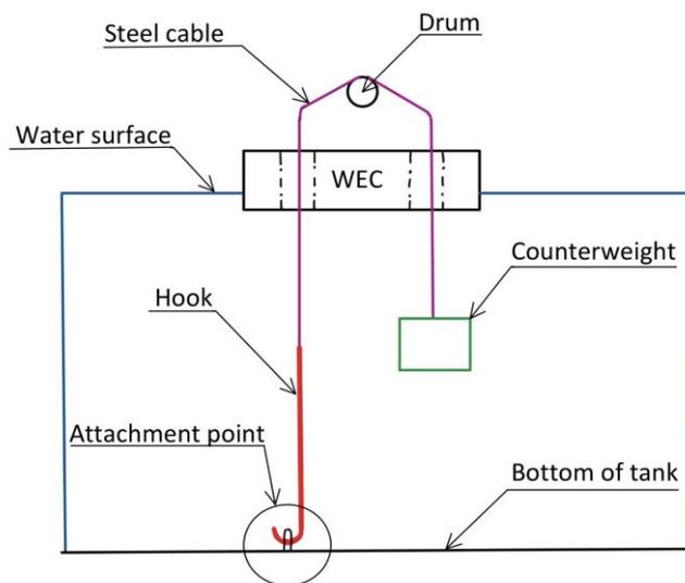
Figure 53 - Illustration of hook and counterweight
