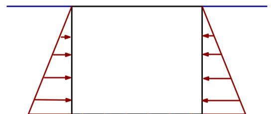
Figure 2 - Hydrostatic Pressure on Submerged Vessel
