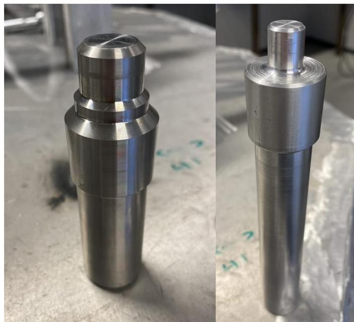
Figure 38 - Steel Axle (Left) and Aluminium Axle (Right)
