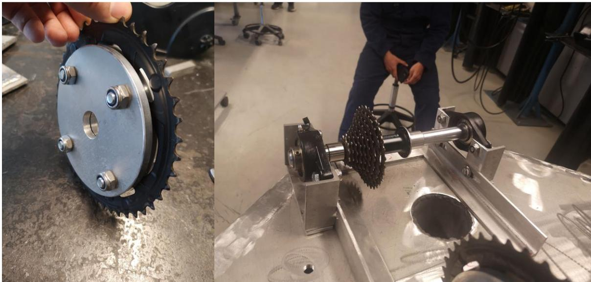
Figure 37 - Sprocket Flange Assembled (Left) & Output-shaft assembled (Right)
