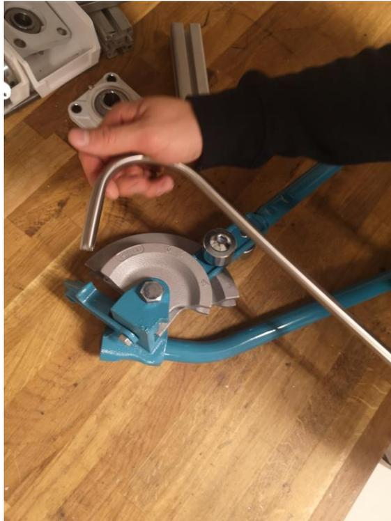
Figure 44 - Bending of steel rod
