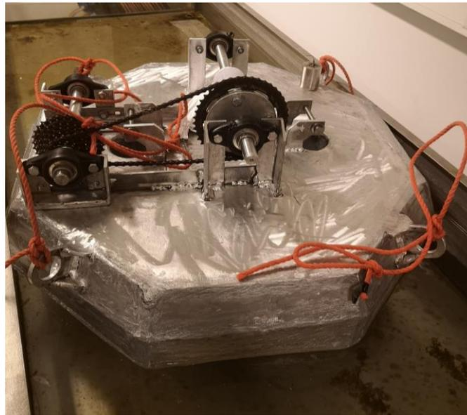
Figure 52 - Balance and leakage test
