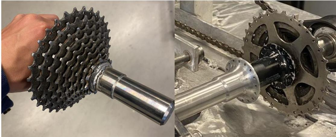
Figure 39 - Steel shaft welded to gears (Left) & Aluminium shaft welded to flange (Right)
