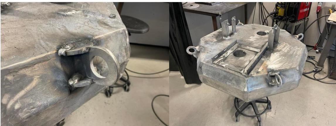
Figure 45 - Mooring attachment (Left) & Placement of Mooring attachment points (Right)
