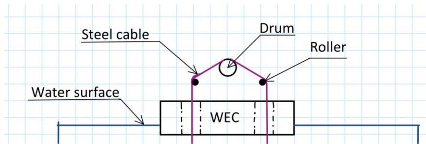
Figure 41 - Illustration of roller
