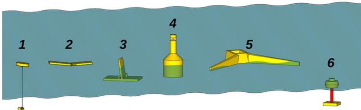
Wave energy generators come in many shapes and sizes. Some designs bob or float on the surface (1, 2, 4) or flip from side to side (3). Another type harnesses energy from waves as they crash onto shore (5). Still others sit near the sea bottom (6).
