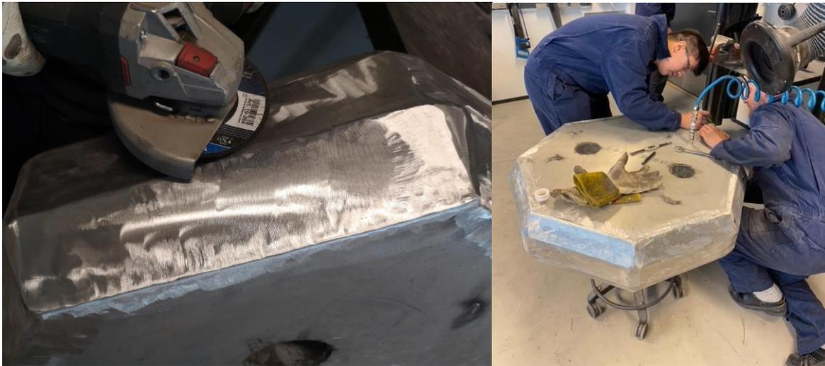
Figure 31 - Grinding Floater (Left) and Pressure Test (Right)
