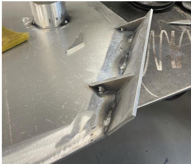
Figure 29 - Orientation Triangles
