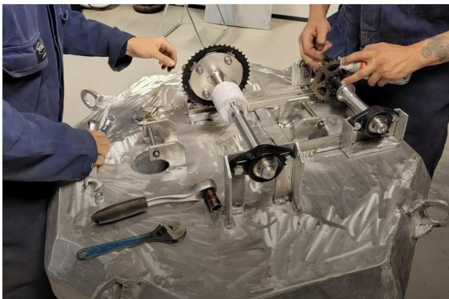
Figure 23 - Lubricating gear with Silicone-penetrant
