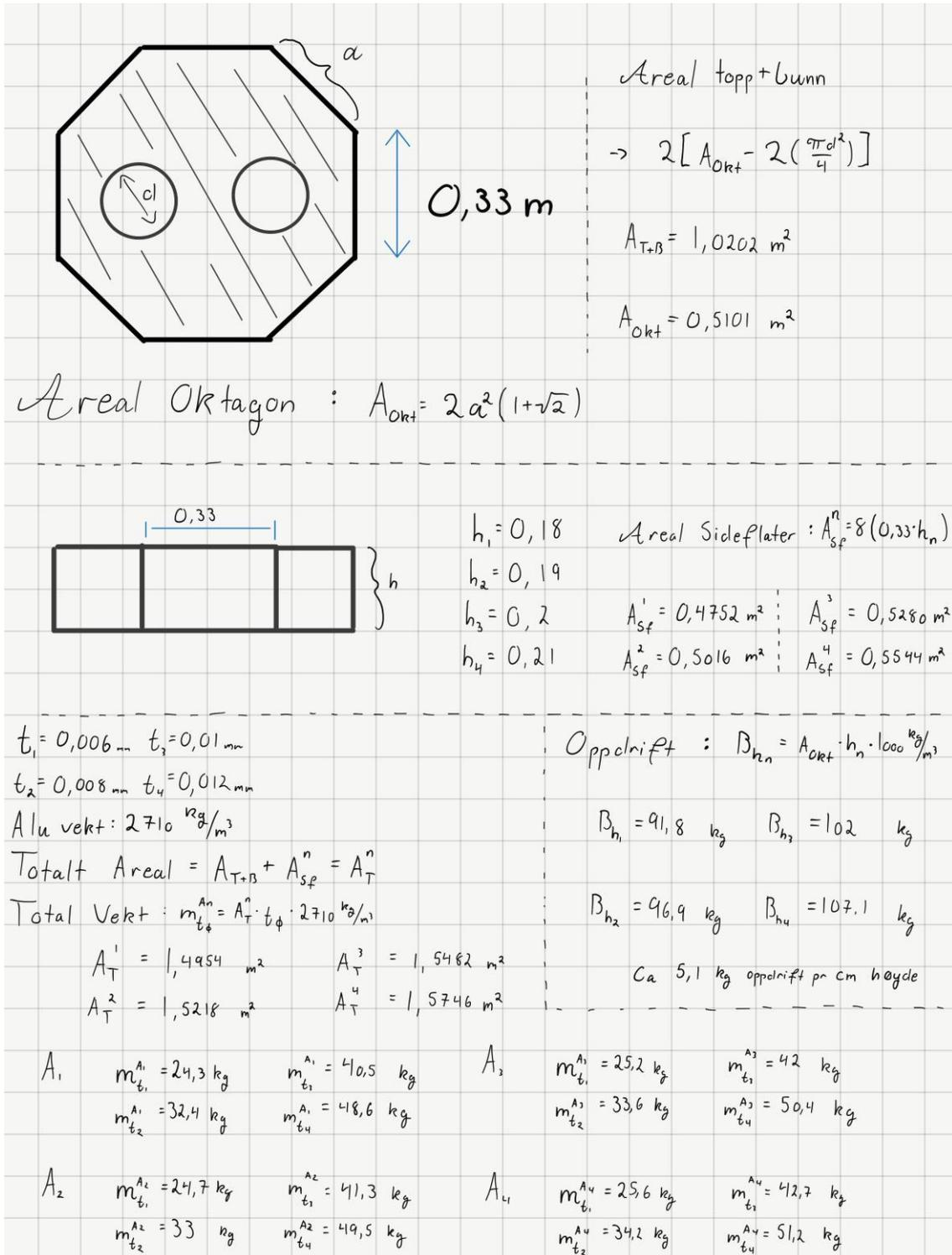
Figure 22 - Buoyancy Calculations
