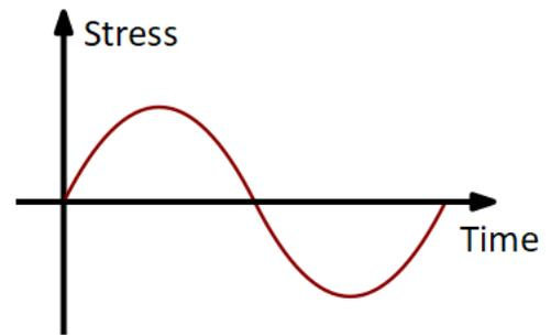
Figure 1 - Stress as a function of Time
