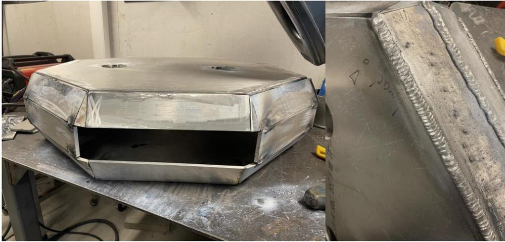
Figure 30 - Floater Unfinished (Left) and Weld Beads (Right)
