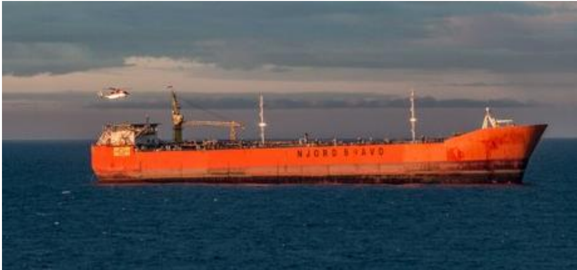
Figure 1: Njord Bravo – offshore oil storage tanker vessel
