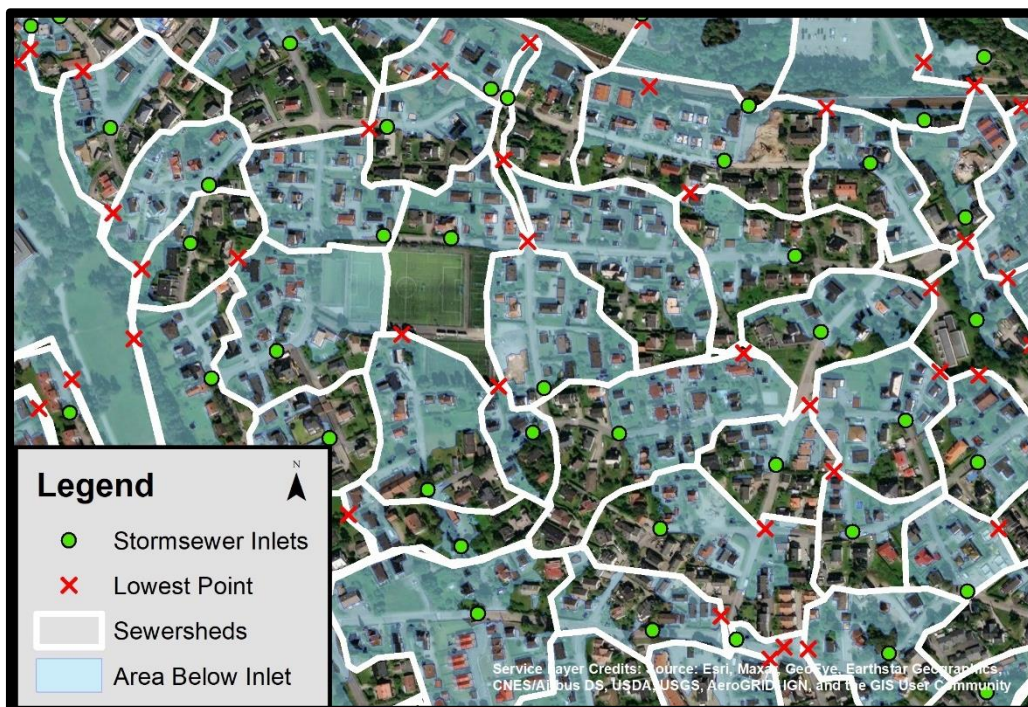
Figure 17: Sewershed inlets rarely corresponded to the lowest point in each sewershed. The area below the inlet (in blue) represents runoff that is neither captured by inlets nor potential ponds surrounding inlets.
