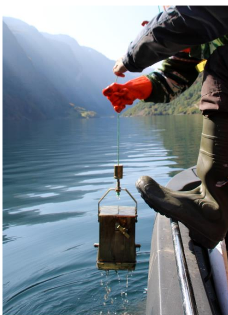
Figure 13: Box corer filled with sediment
