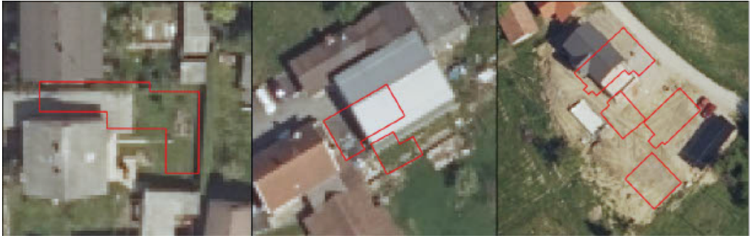
Figure 4: Examples of incorrect building footprints. The most typical errors are footprints that cover meadows, fields and shadows. Examples of partially overlapping footprints and building are un useful.
