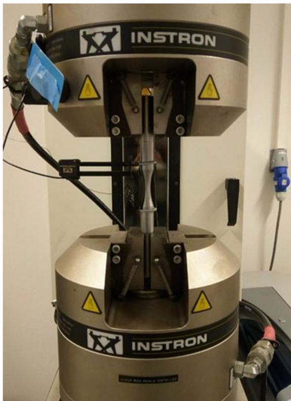
Fig. 10 Mounting of longitudinal extensometer
