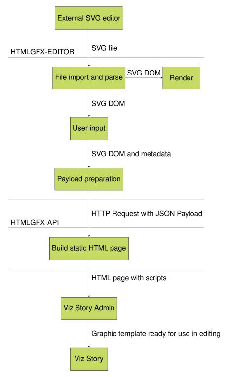
**Figure 4.1.1-1:** The data pipeline of the project.
