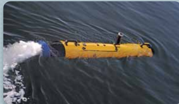
The Bluefin-9's thruster enables speeds of up to 5 knots
