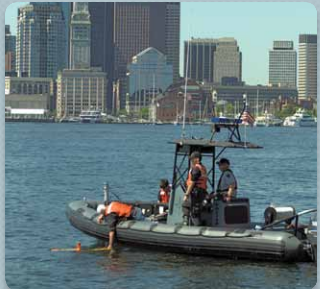
The Bluefin-9 can be easily launched and recovered from a RHIB
