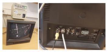
Picture 3: a) Manitar/video and videoprinter. b) Position of different cables (video in, video aut) in monitor when the system is connected.
