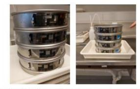
Picture 2: a) The set-up of the sieves, mesh sizes (from the top): 2 mm, 250 µm, 125 µm and 63 µm, b) sieves are placed in a plastic tray in case of spilling of the samples.
