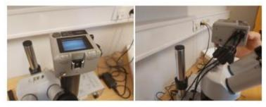
Picture 2: a) Camera mounted on the stereamicroscope. b) Position of the different cables when the system is connected.
