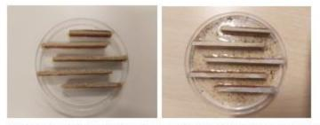
Picture 4: Counting chamber. Each line is suited to the 12X magnification. a) Empty and cleaned. b) Holding a subsample. This density of the particles in this sample is easy to investigate, but one may use a somewhat higher density of particles
