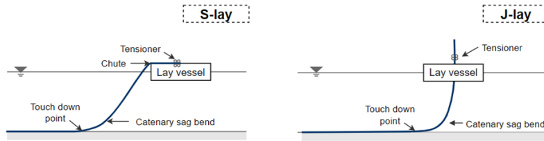
Figure 3. Deployment methods: S-lay and J-lay [19].
