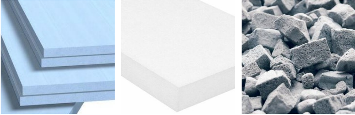
Figure 13: The insulation types of the slab on ground concepts. XPS to the left; Source: (Isodren, n.d.), EPS in the middle; Source: (Glava, n.d.-d) and Glasopor to the right; Source: (Glasopor, n.d.-a).
