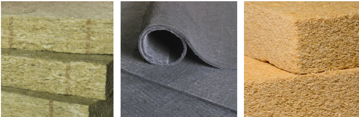
Figure 11: The insulation types of the roof concepts. Stone wool to the left; Source: (Rockwool, n.d.), Aerogel in the middle; Source: (Glava, n.d.-a) and wood fiber to the right; Source: (Hunton Fiber, n.d.-a).
