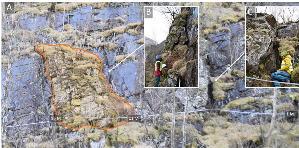
Figure 11: (A) Showing the first part of the structure line located in the lower left area of the rock wall at Site 1, with the unstable area marked in orange. (B) Me (Isak) writing down dip and dip direction measurements along the structure line situated to the right of the unstable area. (C) A large opening in the rock wall using Paula (supervisor) for scale.
