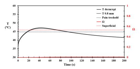
**Figure 6.** The basal layer and 0.8 mm depth skin temperature, and the corresponding damage integral development, versus time for Case 1.
