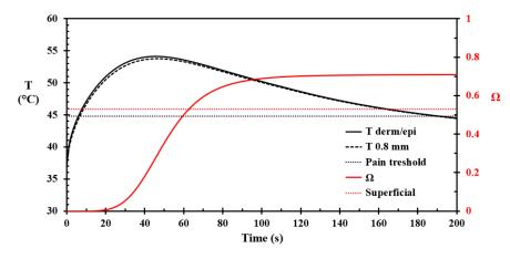
**Figure 9.** The basal layer and 0.8 mm depth skin temperature, and the corresponding damage integral development, versus time for Case 4, i.e.,  $4.0 \text{ kW/m}^2$ , as the flare heat flux to the most exposed point at the pavement.
