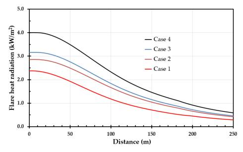
Figure 4. Net maximum flare heat radiation along the pavement for Cases 1, 2, 3, and 4, Table 2.
