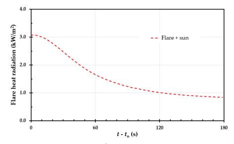
**Figure 5.** The total (flare +  $700 \text{ W/m}^2$  solar radiation) heat flux as a function of time to a passerby evacuating from the most exposed area at a speed of 2 m/s (based on data for Case 1, Table 2).
