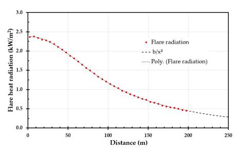
Figure 3. Net maximum flare heat radiation along the pavement for Case 1, Table 2.
