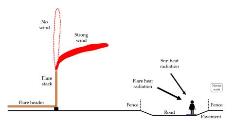
Figure 1. Principal sketch of flare flame heat exposure in varying wind conditions.
