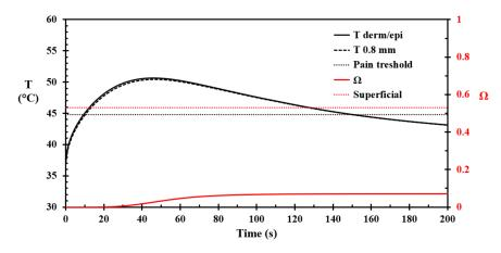
**Figure 8.** The basal layer and 0.8 mm depth skin temperature, and the corresponding damage integral development, versus time for Case 3, i.e.,  $3.16 \text{ kW/m}^2$  as the flare heat flux to the most exposed point at the pavement.
