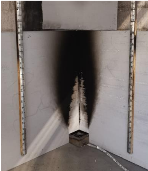
Figure 15 Experimental set-up for propane fire for two-sided boundary A) small-scale B) medium scale
