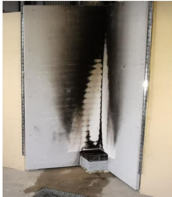
Figure 19 Experimental set-up for heptane fire for one-sided boundary A) small-scale B) medium scale
