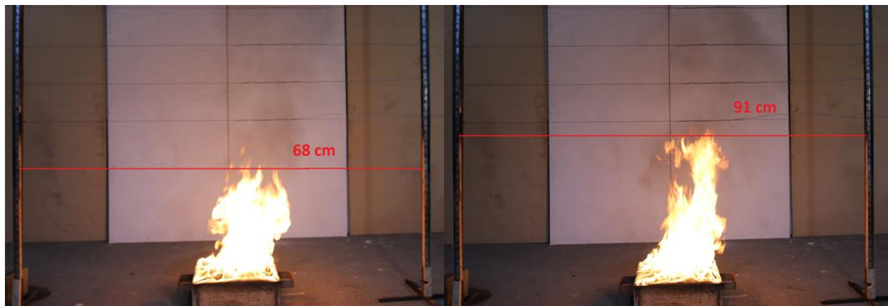
Figure 22 Open mean flame height for medium scale propane fires for A) 76 kW and B) 114 kW.
