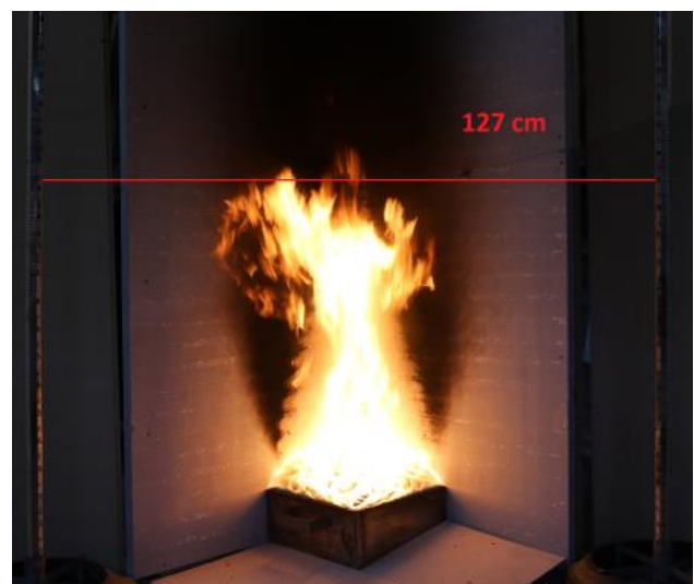
Figure 26 Two-sided boundary surface fire for medium scale propane fires for A) 76 kW and B) 114 kW.
