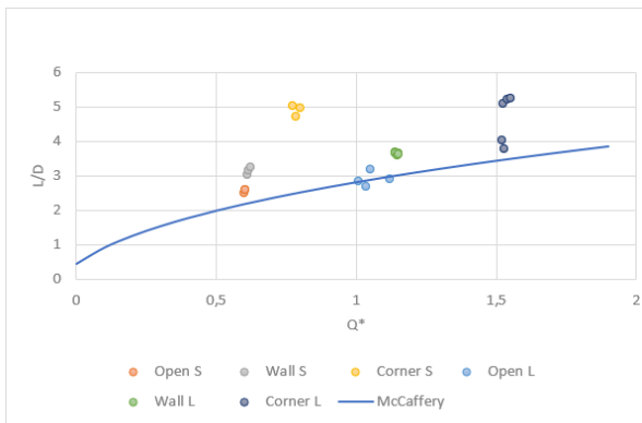
Figure 32 Dimensionless flame height, L/D , as a function of dimensionless energy release rate, \dot{Q}^* , for heptane A) result from small- and medium-scale experiments for all configuration containing heptane B) the average result from small- and medium-scale experiments for all configurations containing heptane.
