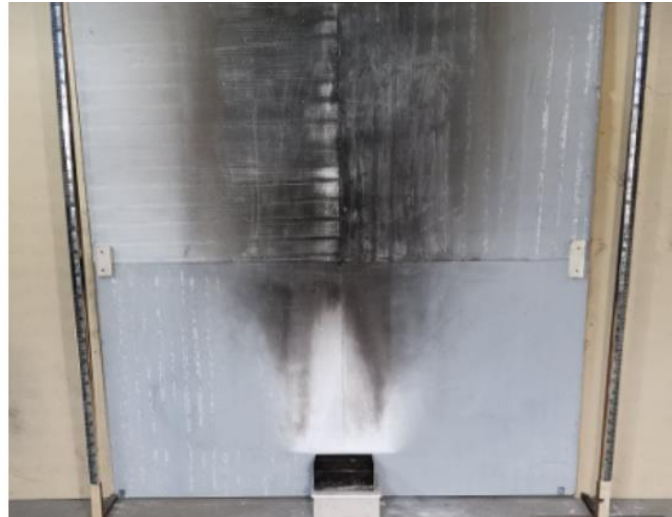
Figure 18 Experimental set-up for heptane fire for one-sided boundary A) small-scale B) medium scale
