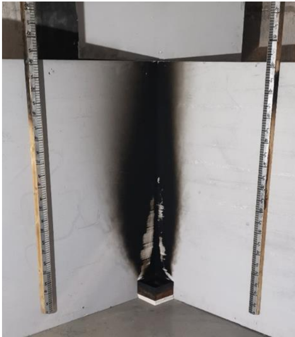
Figure 19 Experimental set-up for heptane fire for one-sided boundary A) small-scale B) medium scale
