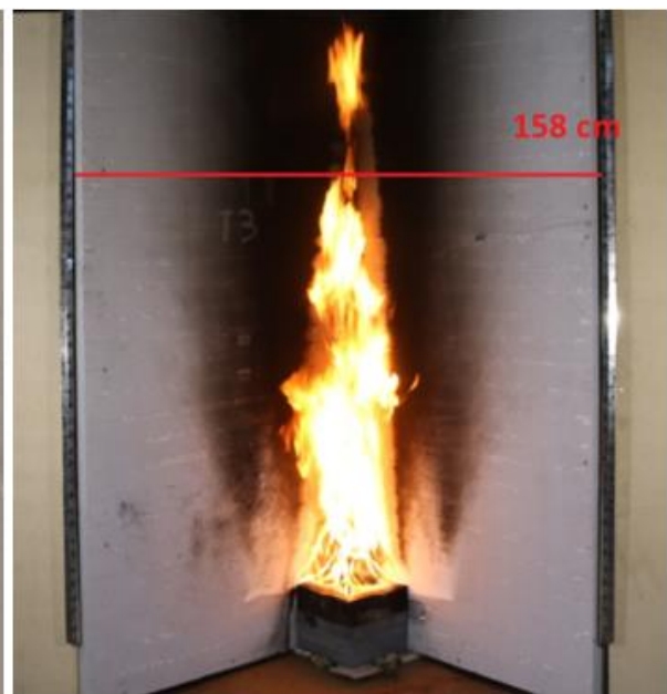
Figure 29 Mean flame height: two-sided boundary surface for A) Small-scale fire and B) Medium scale fire using heptane
