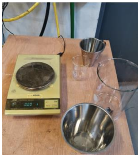
Figure 16 Weight scale used to measure the amount of heptane needed and the measuring cups used to measure the amount of water and pour the liquid in the pan.
