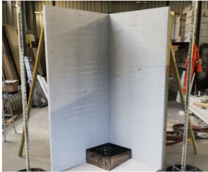
Figure 15 Experimental set-up for propane fire for two-sided boundary A) small-scale B) medium scale
