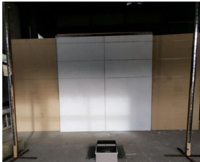
Figure 17 Experimental set-up for heptane fire for free burn A) small-scale: pan is placed approximately 1 meter from the closest wall B) medium scale: pan is placed approximately 2 meters from the closest wall.
