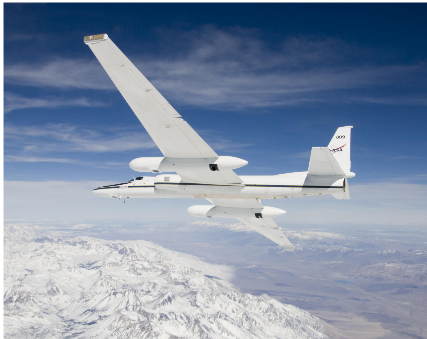
Figure 1: An ER-2 in flight. Earlier versions of the ALOFT project has resided in the pod under the right wing. Pictured by NASA
