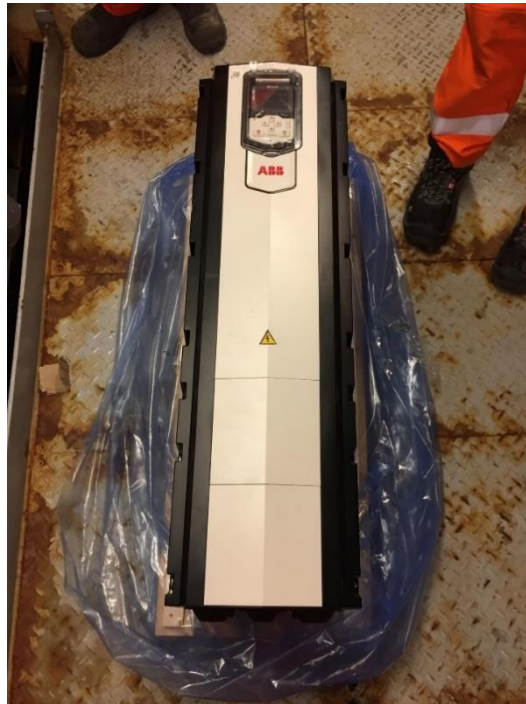
Figure 7. Unpacking the ABB ACS880 VFD.
