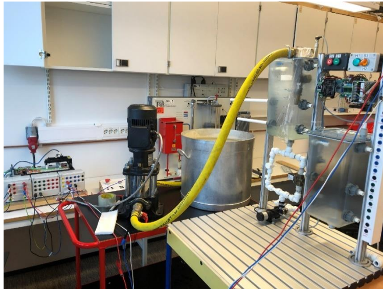
Figure 30. Testing rig to test VFD software.
