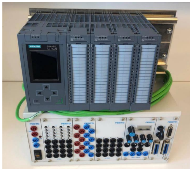
Figure 29. Siemens S7-1500 PLC.
