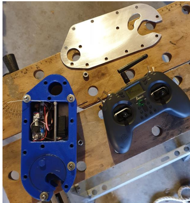
Figure 4.7: Actuator connected to RC receiver Figure 4.8: Assembly of the components
