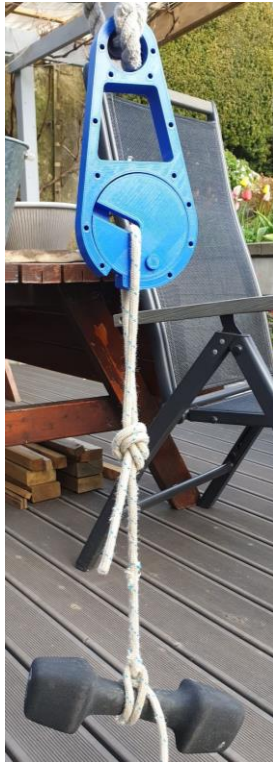
Figure 4.4: Testing release mechanism with 4kg load Figure 4.5: First 3D prototype
