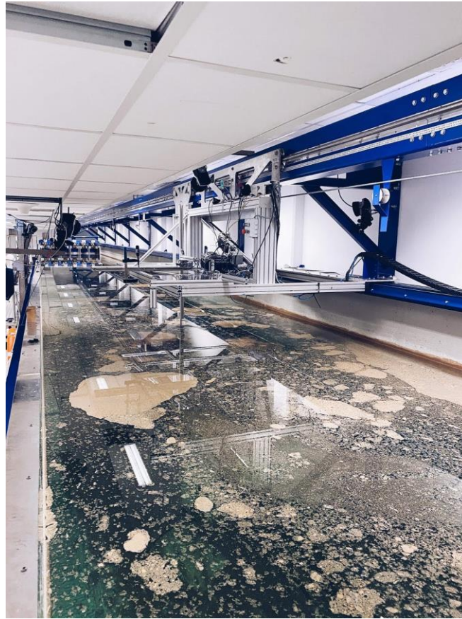
Figure 3-1: Experimental tank at the MarinLab with the carriage
