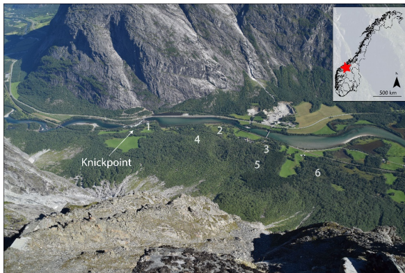
Fig. 1 Photograph of the study site taken in 2016 from the top of the Mannen rock-slope instability. The photo features the transition from a wide cross section to a strongly confined valley section. A knickpoint in the river's long profile, visible due to rapids, is created by a rock-slope failure event. Numbers 1-6 represent rock-slope failure deposits hidden under the forest.
