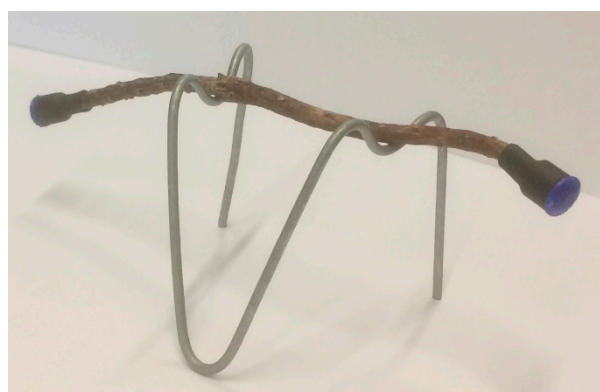
Figure 1. Sample holder and test specimen ready for climate chamber drying.
