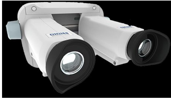
Figure 1: fMRI goggles. The fMRI goggles created by NNL as a part of the Visual Systems HD solution, NordicNeuroLab, 2020. Available from: https://nordicneurolab.com/nordic-fmri-solution/
