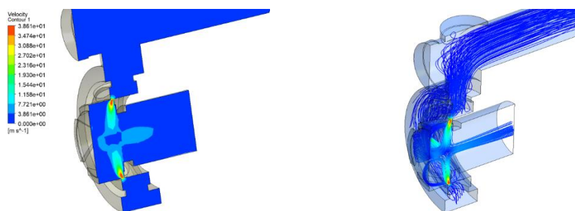
Fig. 3. Velocity distribution (left side, in m/s) and pathlines (right side) for the part with spool controlled by solenoid
