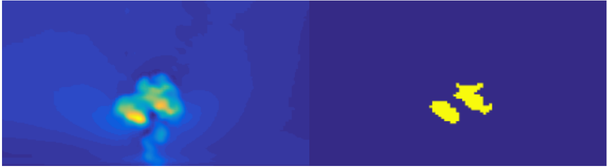
Figure 22 - The picture on the left is the plotting of the original subtracted matrices. While the picture on the right is the result of plotting the binary matrices. Both pictures are vertical slices showing the cross section of a bent over plume at 250 meters downstream from the source. Though not considered in this report, note the appearing counter rotating vortices [4] [58]
