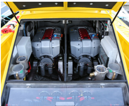
Engine room (showing 2 x Steyr installed)
