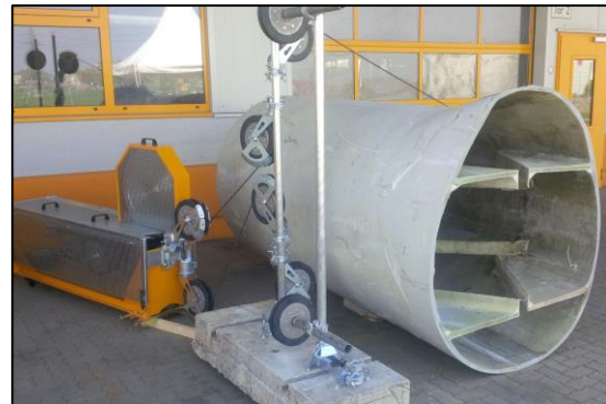
Figure 34: Mobile unit with temp. support structure [92]
