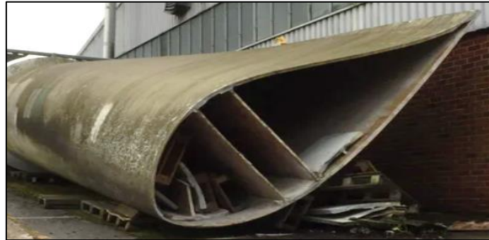
Figure 9: Cross-section wind turbine blade [31]
