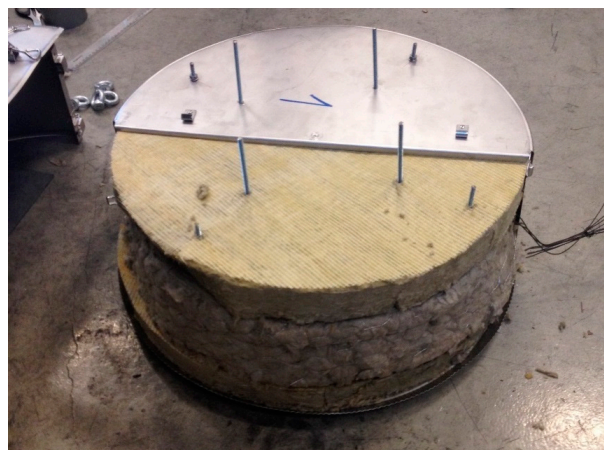
Figure 6. Mockup nearly ready for fire exposure. (Thermocouples exiting to the right).
