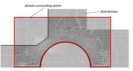
Fig. 5. Overset mesh model for safety valve presented in Fig. 1.
