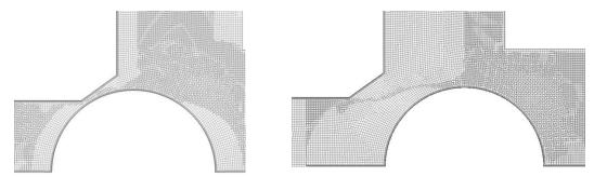
Fig. 7. Grid interface between two fluid domains.
