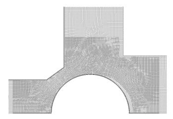
Fig. 6. Overset mesh model for safety valve presented in Fig. 1.
