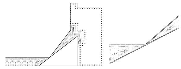
Fig. 4. Lattice nodes for direct operating relief valve (Domagala, 2016)
