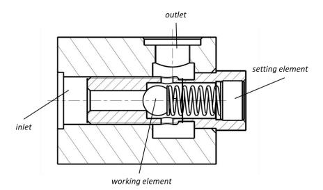
Fig. 1. Simplified drawing of direct acting relief valve
