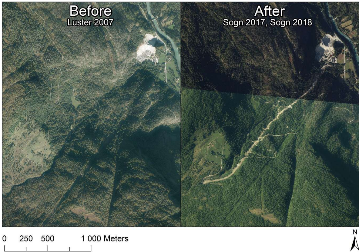
Figure 17: Røneid power plant in Luster municipality shows a clear scar after the power plant is built. The main part of this scar in the forest is the deforestation of the waterway path and the roads. The area usage of the waterways and roads is estimated by the application documents to be 34,8 daa. Images collected from norgebilder.no. The caption on the figure refers to the layers from norgebilder.no and is the name of the layers containing the aerial photos. The first part of the caption refers to the area contained in the layer and the last part refers to the year the aerial photos were created i.e. Sogn 2018 contains aerial photos from the area of Sogn from 2018.
