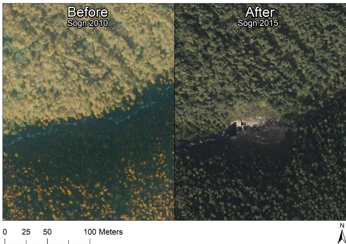
Figure 12: Due to the construction method of the waterways the intake is also quite well hidden. It has a permanent area usage of 0,9daa. Because there is no deforestation from building waterways the intake is hidden in a forested valley and not visible from the valley. Images collected from norgebilder.no. The captions on the image refers to the layer on norgebilder.no used in the image. In figure 12 the layers used is Sogn 2010 and Sogn 2015, the first part of the name Sogn refers to the area mapped in the relevant layer. The second part of the caption refers to the year the aerial images was taken.
