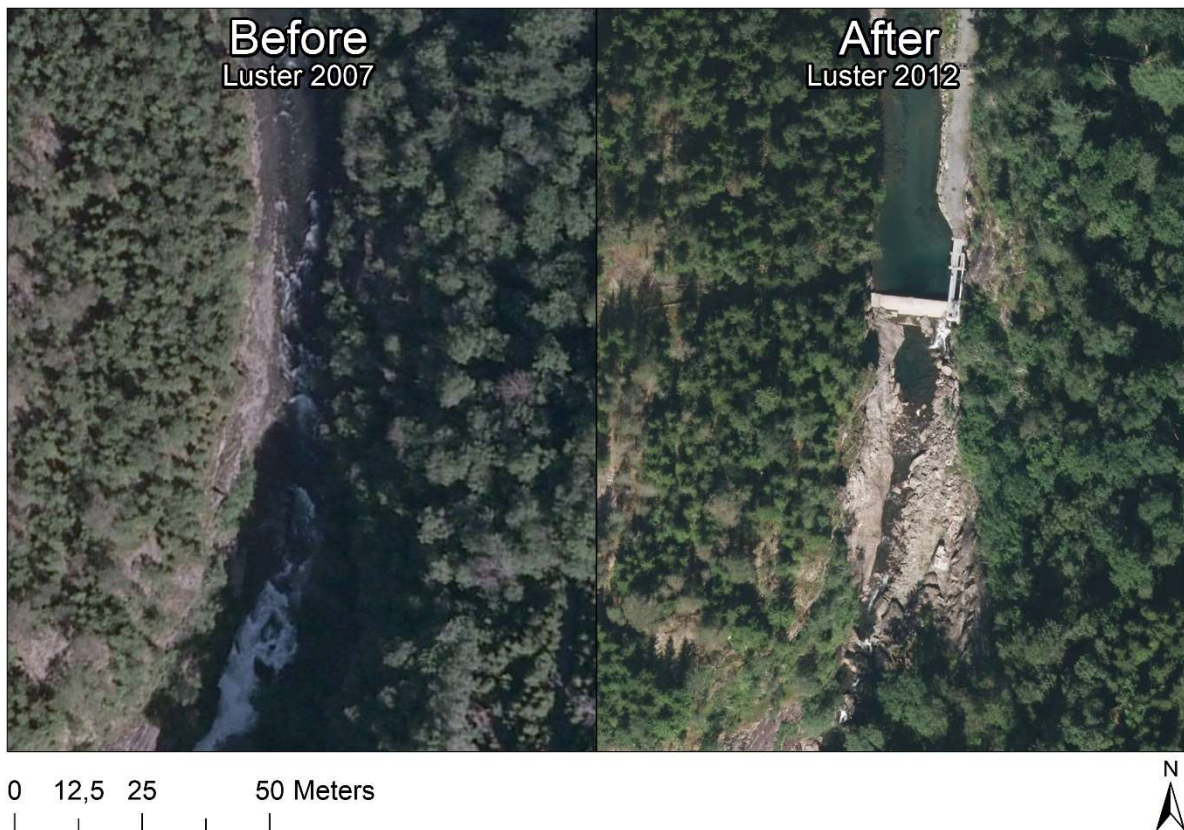
Figure 15: The dam makes a new reservoir on the upside of the dam and heavily reduces the water flow downstream. The application does not give a number for how much area is used for the intake. Images collected from norgeibilder.no. The caption on the images refers to the layers from norgeibilder.no. Luster 2007 and Luster 2012 is the layers used. The first part of the caption is the area the layers contain, here it contains aerial photos from Luster, Sogn & Fjordane. The second part is the year the aerial photographs were taken.
