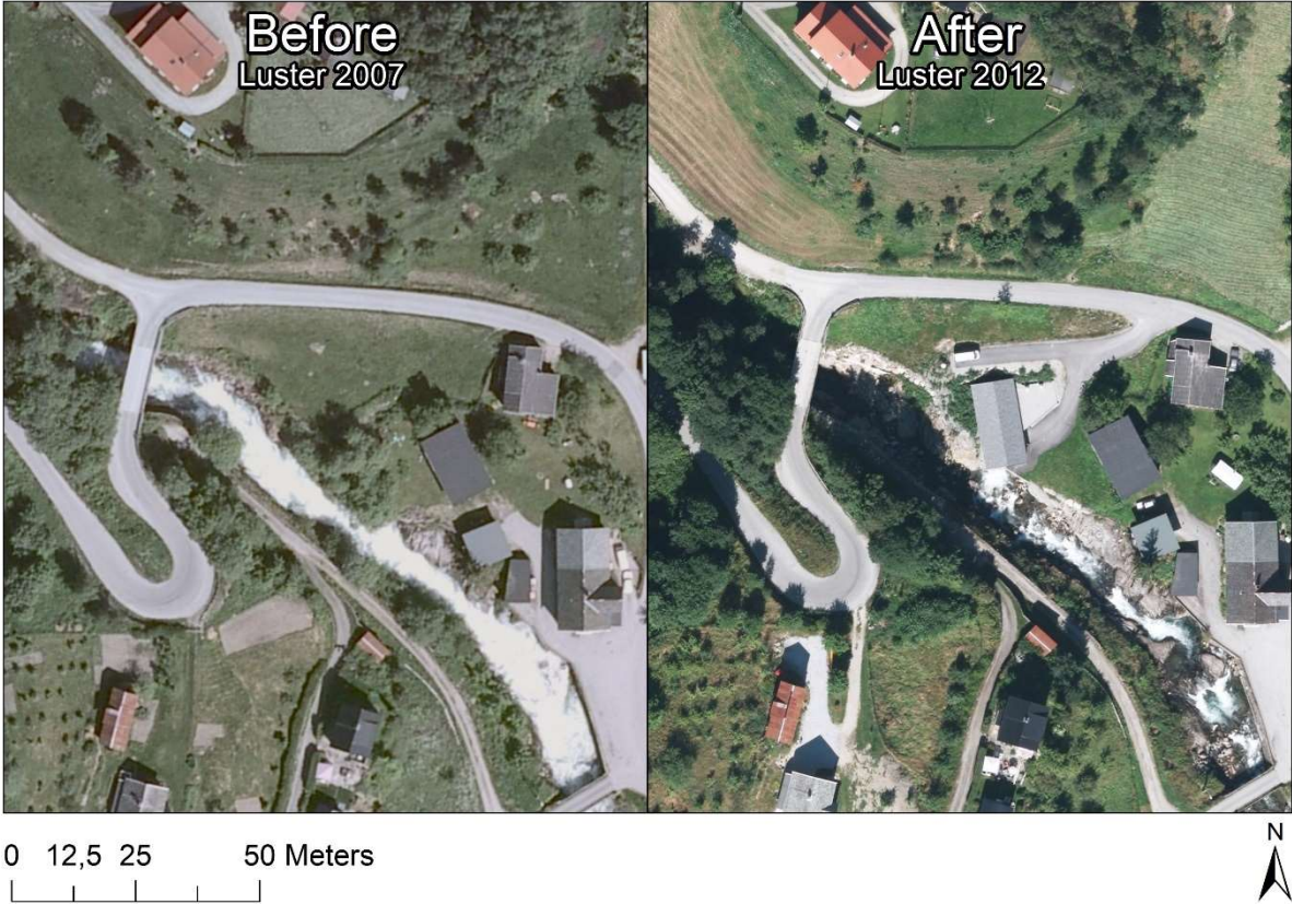
Figure 16: The powerhouse at Kvåle power plant is located in the middle of the small village of Luster and blends in well with the surrounding buildings. The powerhouse contains 2 Francis turbines and have a maximum capacity of 4,6 MW. The powerhouse is estimated to use 0,1 daa. Images collected from norgeibilder.no. The caption on the images refers to the layers from norgeibilder.no. Luster 2007 and Luster 2012 is the layers used. The first part of the caption is the area the layers contain, here it contains aerial photos from Luster, Sogn & Fjordane. The second part is the year the aerial photographs were taken.
