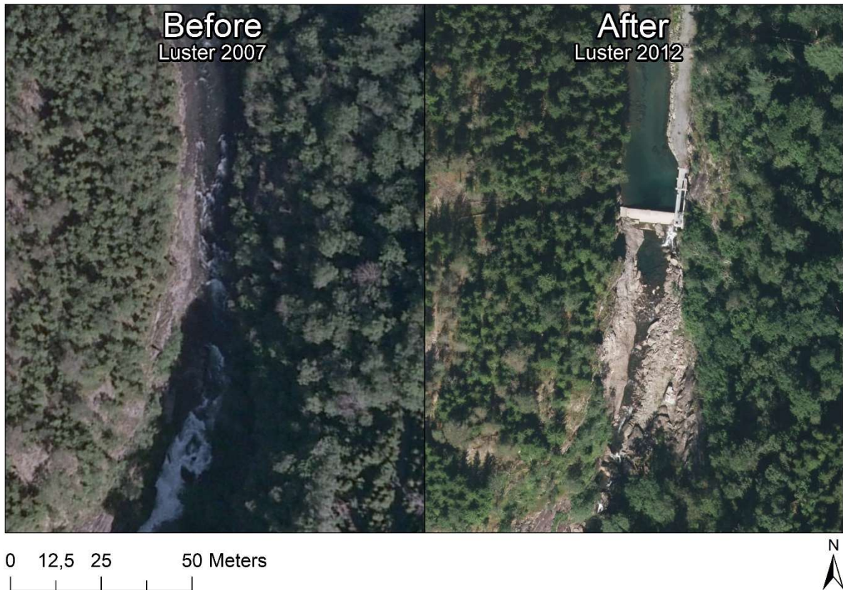
Figure 2: Example of a dam built in Luster municipality in connection with the Kvåle power plant described later in the thesis. It is clearly visible that the dam alters the water flow downstream and the amount of water above the dam. Pictures collected from norgeibilder.no. The caption on the images Luster 2007 and Luster 2012 refers to what layers of aerial images from norgeibilder.no were used. Luster refers to the area the specific layer covers and 2007/2012 refers to the years the layers were created.
