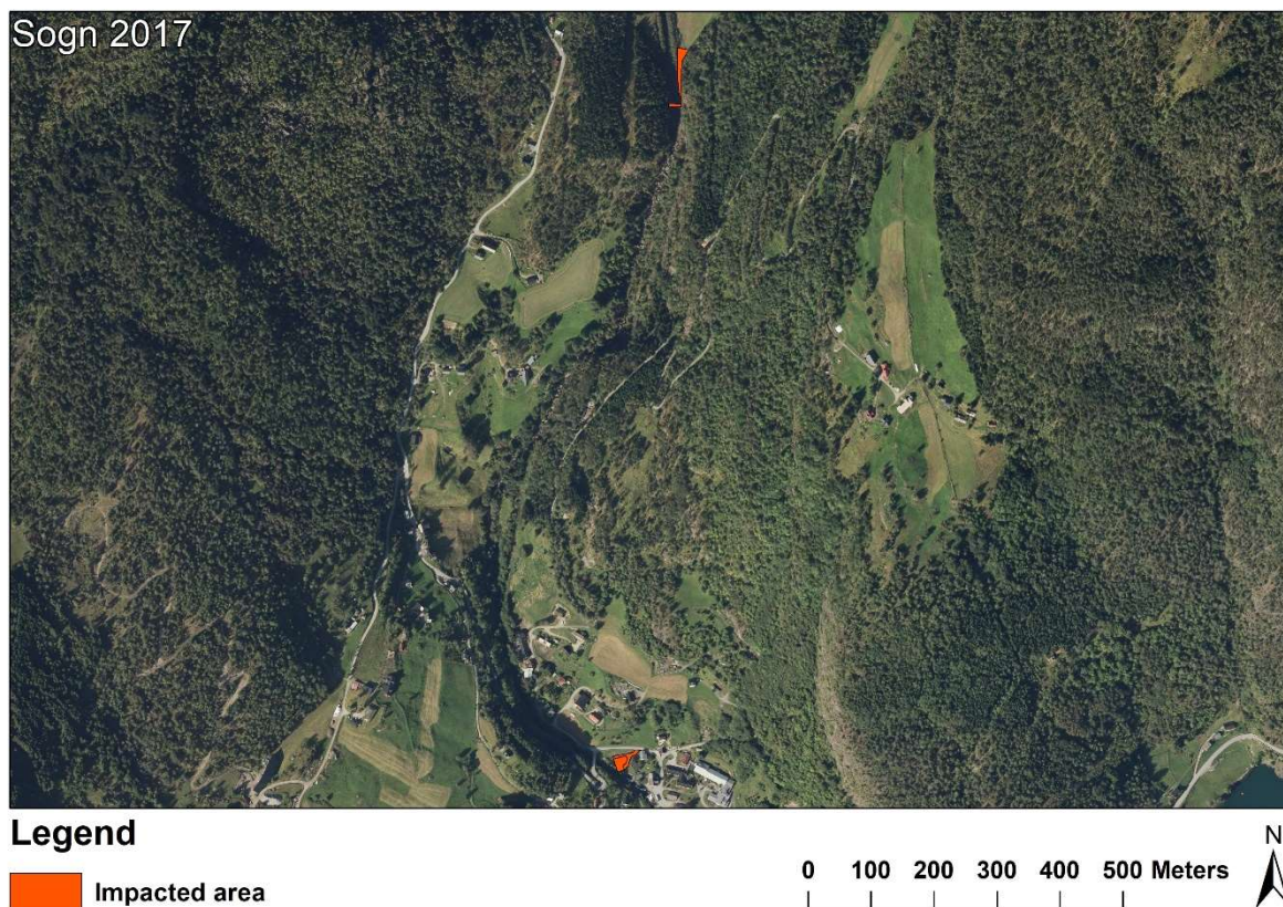
Figure 24: The image shows the impact due to the construction of the Kvåle power plant in Luster municipality. The impacted area is 1,3daa and is marked by the orange fields. Images collected from norgebilder.no. The caption Sogn 2017 refers to the layer from norgebilder.no used in the figure. The name of the layer refers to the area in the layer and the year the photography's was taken.
