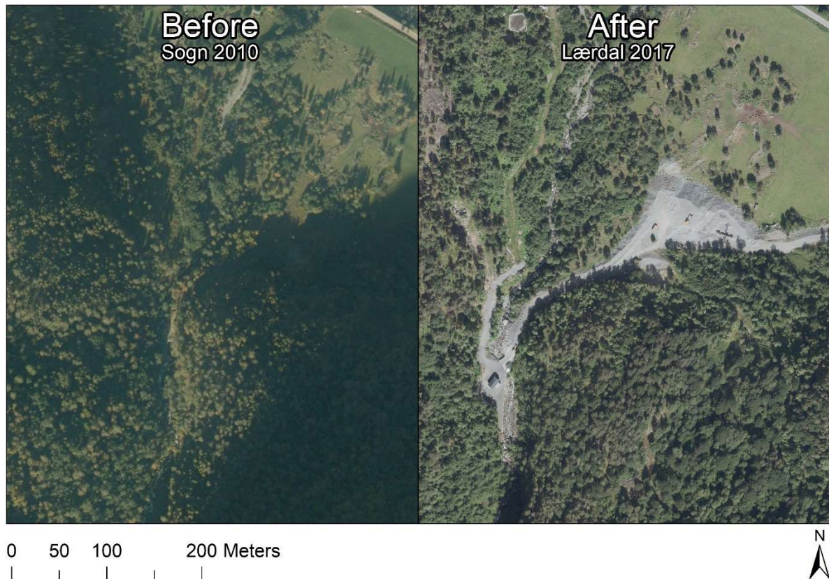
Figure 13: At Kvemna power plant the application estimates that the powerhouse and the roads connected to it have a total area usage of 3,2daa. The powerhouse contains a 5MW Pelton turbine. One can clearly see the impact on the local environment by the powerhouse, roads and quarry in connection to the power plant. Images collected from norgeibilder.no. The captions on the image refers to the layer on norgeibilder.no used in the image. In figure 13 the layers used is Sogn 2010 and Lærdal 2017, the first part of the name Sogn and Lærdal refers to the area mapped in the relevant layer. The second part of the caption refers to the year the aerial images were taken.
