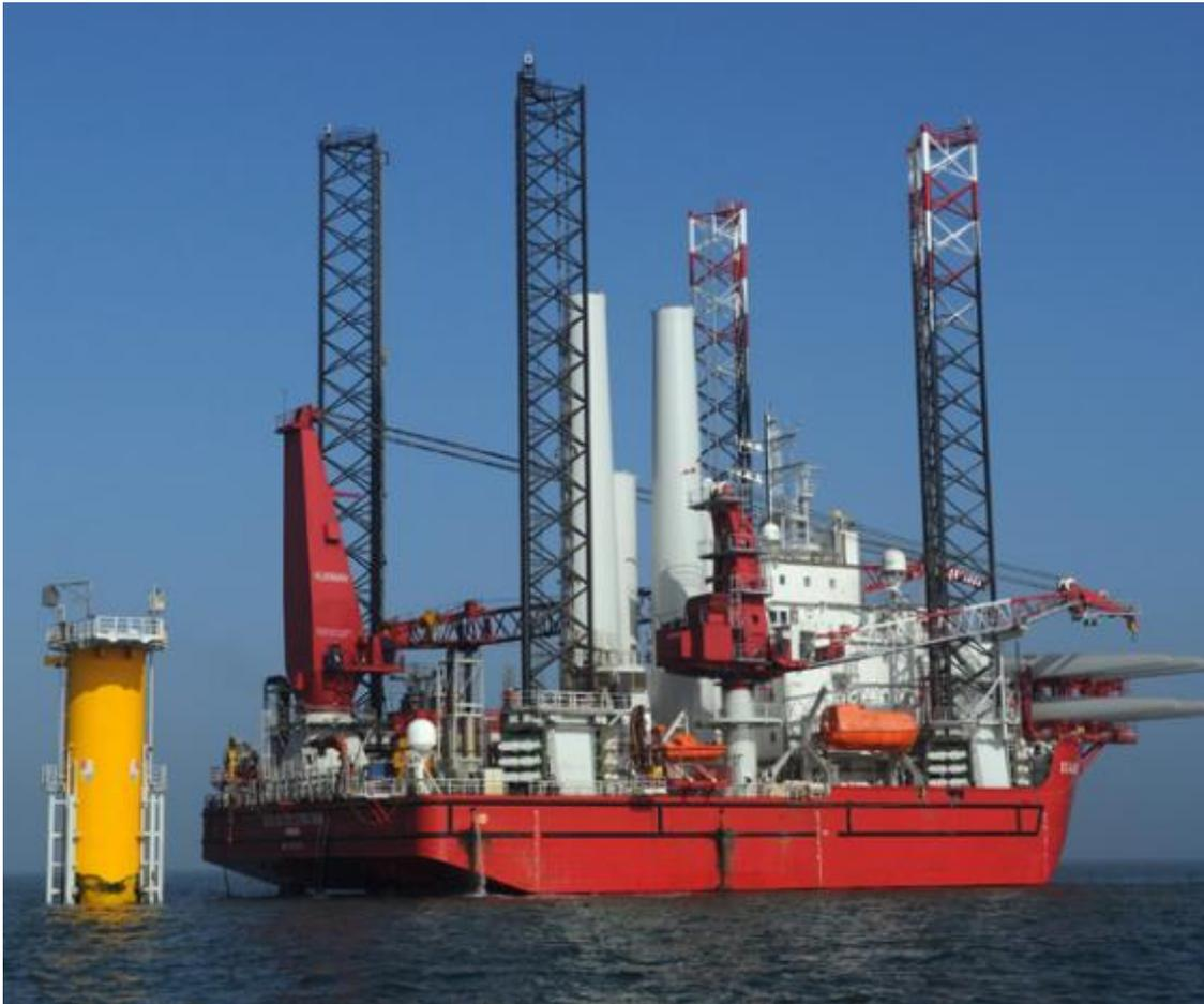
*Figure 9: Jack-up vessel "Seajacks Leviathan" loaded with tower and blades, next to a monopile fitted with the yellow transition piece [3].*
