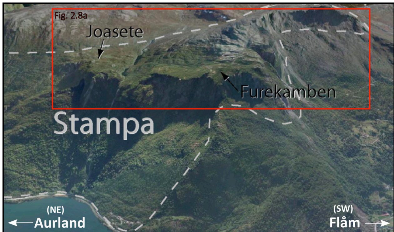
Fig. 2.7 – Photograph showing the extent (white stippled line) of the area (11 km 2 ) affected by active gravitational deformation. The frontal cliff between Joasete and Furekamben has the highest movement rates, with eight potential failure-scenarios (Fig. 2.8a). Modified after Böhme et al. (2013).
