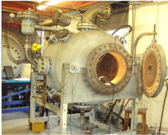
Figure 12: Leeds ISO 1 m 3 vessel [59]
