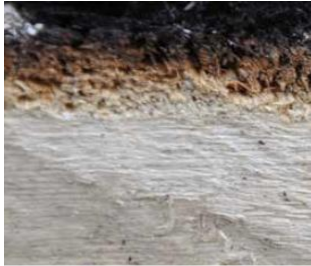
Figure 24 Cross section of a charred CLT element [14]
