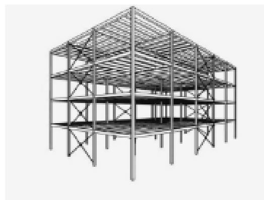
Figure 12 Post and beam- Skelet system [36]
