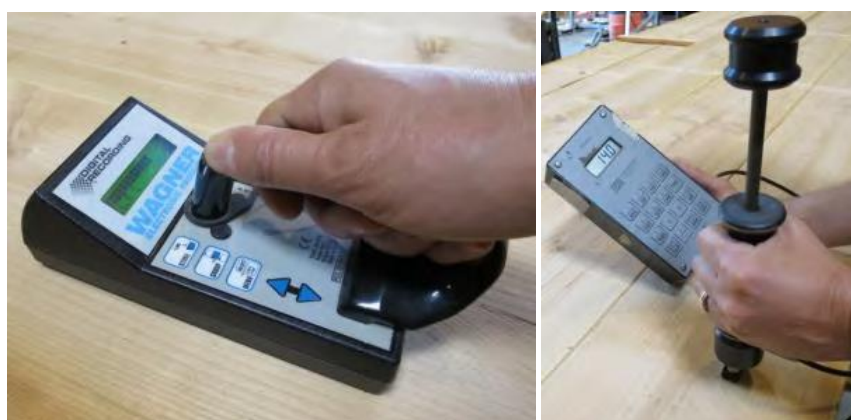
Figure 30 Measuring wood moisture content using a capacitance-based meter (left) and a resistance-based meter (right) [21]
