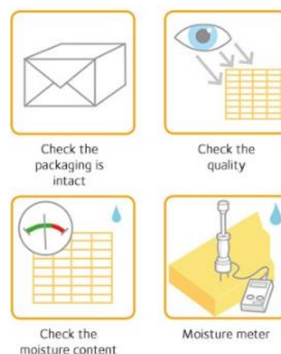
Figure 35 Good practices in material delivery [58]
