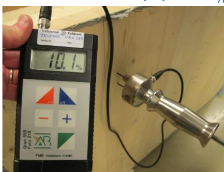
Figure 28 Measuring MC of a CLT panel using a resistance method device [44]
