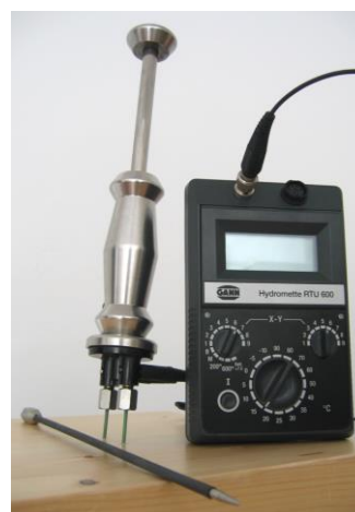
Figure 26 Commercially available device using the resistance method [23]
