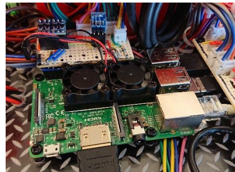
Figur 22: SBC Raspberry Pi
