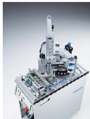
Figur 2 - Festo Storing station, in and out
