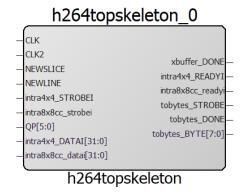
Figure 9. HardH264 IP's top level
