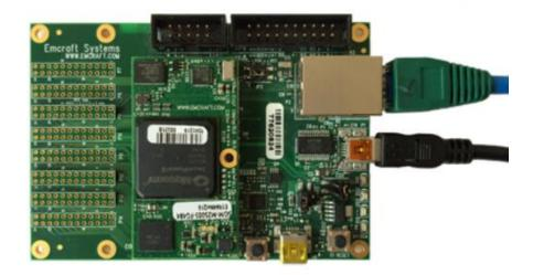
Figure 6. Smartfusion2 System-on-chip Starter Kit
