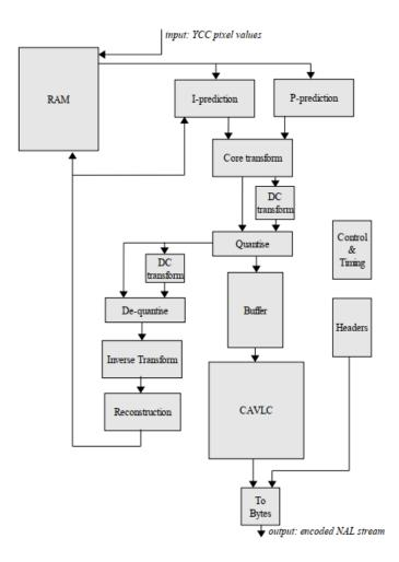
*Figure 8. Principal components in H.264 encoder*
