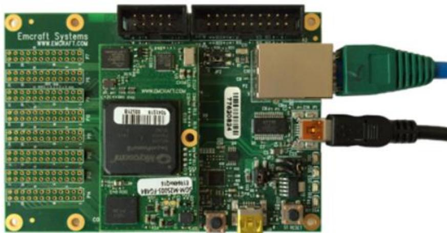
*Figure 6. Smartfusion2 System-on-chip Starter Kit*
